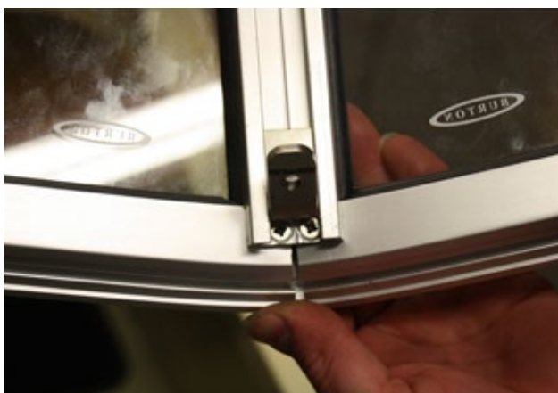
Mount the mounting bracket.
