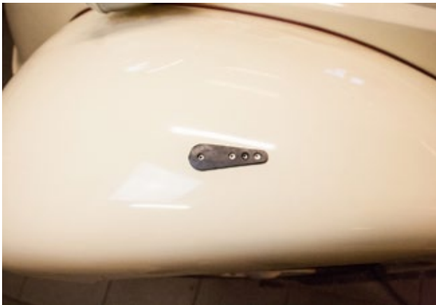
Mount the mounting plate
