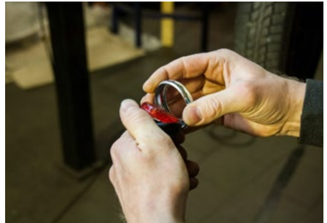
Disassemble the reflector.
