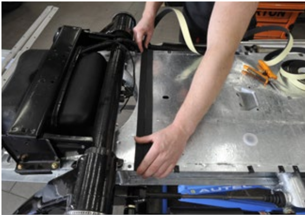
Fit double chassis tape to the rear.
